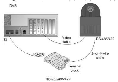
Connecting a dome camera to a recorder.
