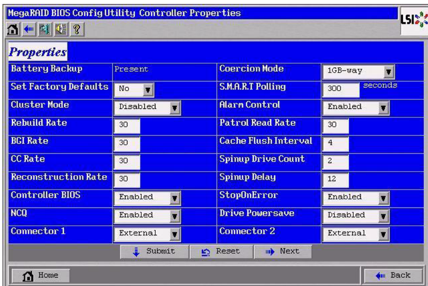
Figure 3.38 Second Controller Properties Screen
