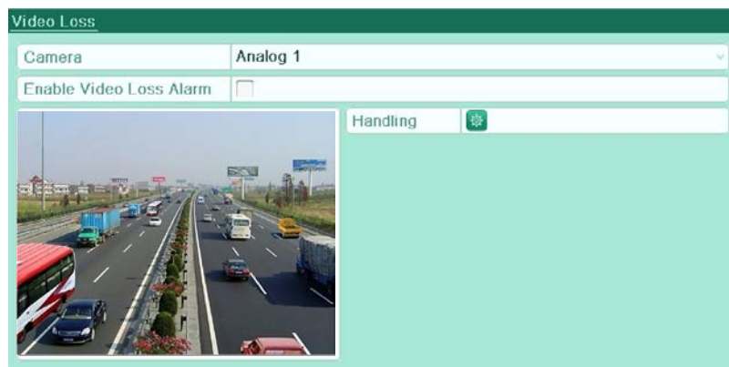
Figure 8.7 Video Loss Setup Interface
