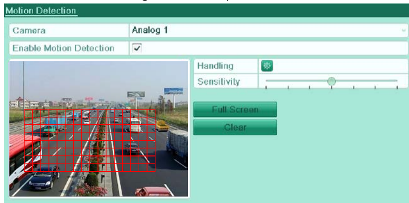
Figure 8.2 Set Detection Area and Sensitivity
