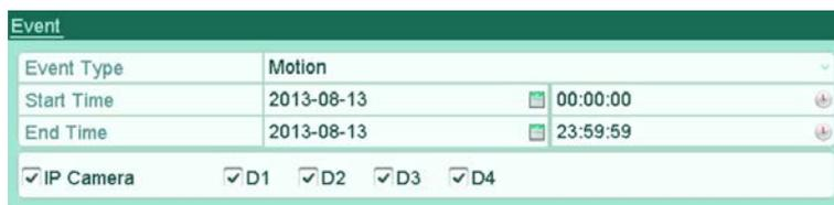
The interface shows an 'Event' search window. It includes fields for 'Event Type' (set to 'Motion'), 'Start Time' (2013-08-13 00:00:00), and 'End Time' (2013-08-13 23:59:59). Below these fields are checkboxes for 'IP Camera' and channels 'D1', 'D2', 'D3', and 'D4', all of which are checked.
