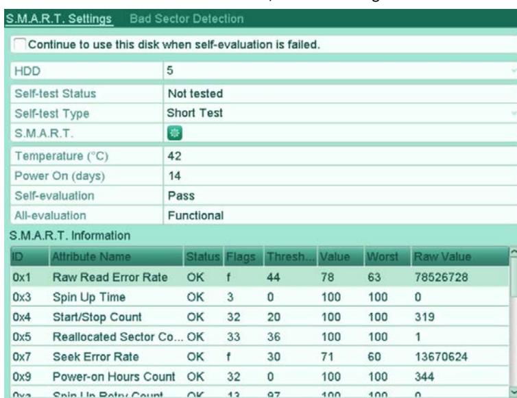
The screenshot shows the S.M.A.R.T. Settings interface. At the top, there are two tabs: "S.M.A.R.T. Settings" and "Bad Sector Detection". Below the tabs, there is a checkbox labeled "Continue to use this disk when self-evaluation is failed." which is currently unchecked. Below this, there is a table with the following data:
