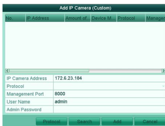
Figure 2. 14 Custom Adding IP Camera Interface
