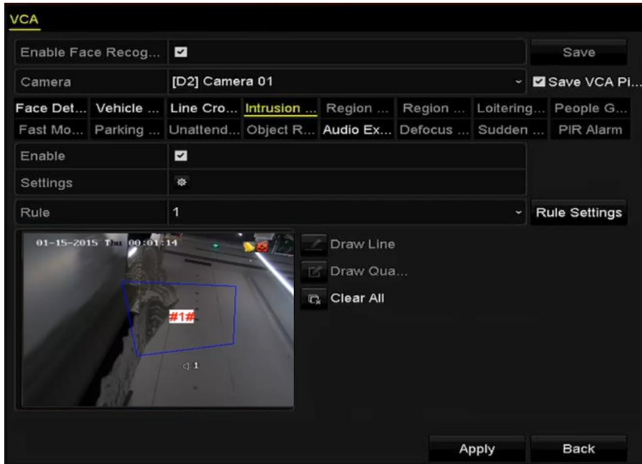
Figure 9. 4 Draw Area for Intrusion Detection
