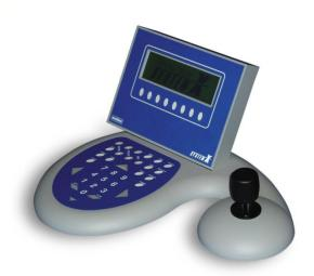
Operating a video matrix should be easy and straightforward. The keyboards for the Ernitec System-X have been designed with that in mind all the way from the appearance of them to the layout of the keys, the functionality and the menu structures. The ergonomically designed keyboards, specially designed for System-X, offers a range of features making the surveillance system very comfortable and precise to control.
