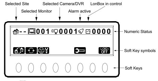
The Escape key  $\bigcirc^{\text{\tiny ESCAPE}}$  can be used to step back through the 'Soft Key symbols'.
