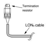
In a bus topology networksegment, two terminations are required, one at each end of the bus. The termination resistors should each be a 105  $\Omega$ , 1/4W type.
