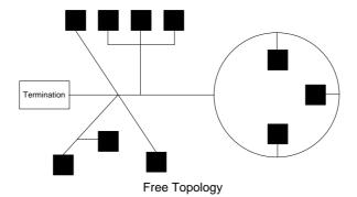
When using free topology, the maximum cable length in one segment is approx. 500 meters, and is calculated adding together all cables used. The maximum number of nodes in one segment is 64. If more that 500 meters, or more than 64 nodes, is required, two or more network segments can be made, using a repeater between each segment.
