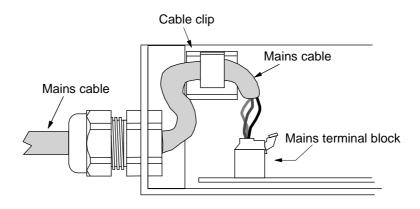
WARNING: Make sure the equipment is earthed; otherwise the over voltage protection will not work! Although both the transmitter and the receiver are earthed no hum bar problems will occur due to the galvanic separation of the video signal in the receiver.
