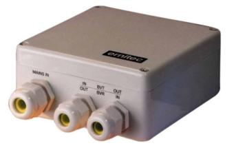
The Ernitec Series 65 is a range of units capable of transmitting colour and black and white video signals on twisted pair cables up to a distance of 1000 m. The Series 65 twisted pair transmission equipment can be used in a variety of applications, such as linking a camera to a matrix, transmitting video from a remote matrix to a main matrix or from a matrix to a remote monitor.
