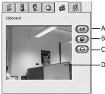
The Clipboard in the Properties window. A. Capture B. Save C. Print D. Captured image
