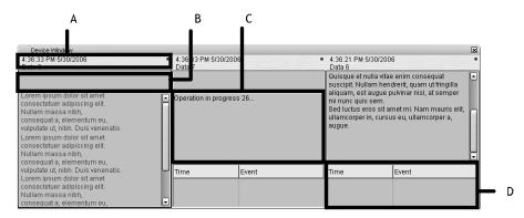
Three text channel views in a device window. **A**. Date, time and name of the channel **B**. Header **C**. Text data list **D**. Custom event list.
