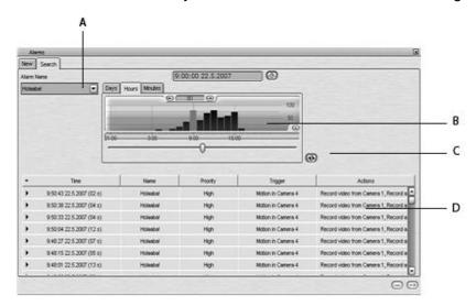
Alarm Search. **A**. List of alarm names **B**. The graph shows the number of alarm events. The selected bar is shown in yellow in the graph. **C**. Refreshes the graph and the list to show the most recent alarms **D**. Alarms generated during the selected time.
