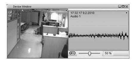
An alarm window with one alarm video view and one alarm audio view. The name of the alarm and the time it was activated are shown in the title bars.
