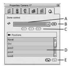
The Dome Control tab of the **Properties** window. **A**. Camera tours **B**. Edit camera tours **C**. Buttons for controlling camera tours **D**. Preset positions **E**. Buttons for adding and deleting preset positions
