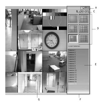
Local monitoring. **A**. Minimize, Maximize and Close buttons **B**. Shows the alarm list **C**. Click to hide the control panel **D**. Click one of these buttons to change how many video views are shown **E**. Available cameras **F**. Control panel **G**. Image area
