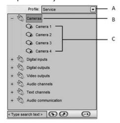
A sample profile on the Navigator pane. A. Profile selection, B. Device groups, C. Devices
