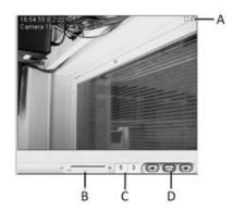
Camera tour window. **A**. The camera tour symbol shows that a tour is running **B**. Slider for changing the dwell time **C**. In seconds, the remaining time this camera will be shown and the time that each camera view is shown (dwell time) **E**. Buttons for manual control of the tour
