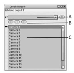
A video output view. A. Saved camera tours B. Camera tour controls C. Shows the selected camera on the monitor
