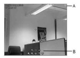
A controlled dome camera. **A**. Dome camera symbol **B**. The zoom, iris, focus and preset controls
