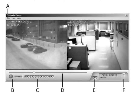
A synchronized media clip from two cameras. **A.** Click **File** and then **Open** to play a different media clip **B**. The green circle and the text **Authentic** show that this clip is authentic. **C**. Playback buttons Information about an audio channel **D**. Playback slider **E**. Mute **F**. Volume
