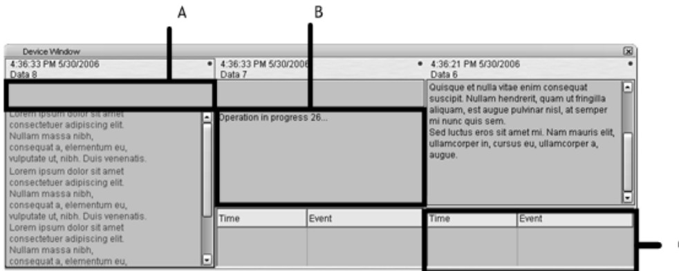
Three text channel views in a device window in Workstation. A. Header B. Text data list C. Custom event list.
