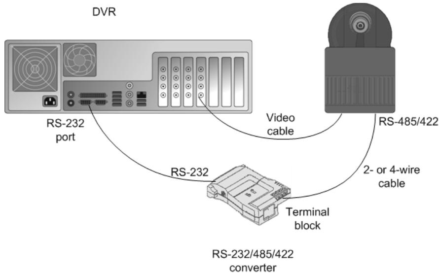
*Connecting a dome camera to a recorder.*
