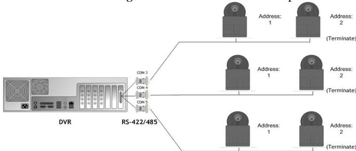
*Using a combination of daisy chained cameras with a multiport serial board*
