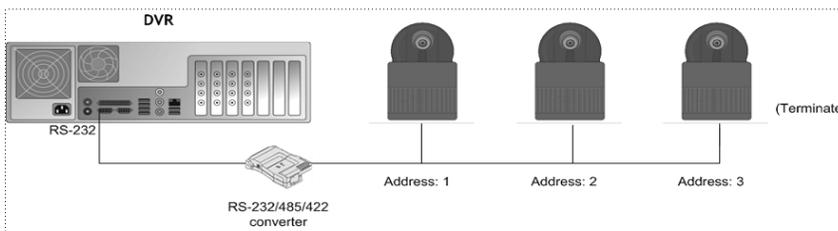
*Using a daisy chain configuration to connect multiple dome cameras*
