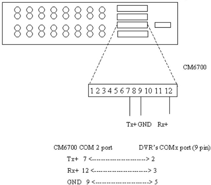
Pin diagram for connecting the Pelco CM6700 Switch to a recorder using a RS-232 connection.
