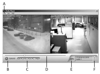
A synchronized media clip from two cameras. A. Click **File** and then **Open** to play a different media clip **B**. The green circle and the text **Authentic** show that this clip is authentic. C. Playback buttons Information about an audio channel **D**. Playback slider **E**. Mute **F**. Volume
