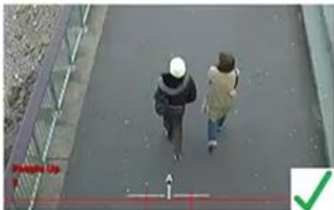
Lower Line and Steeper Angle Greater Accuracy
