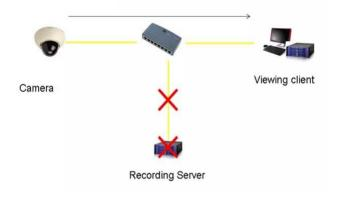
It is possible to get the direct stream from the camera to the client also when the recording server connection is OK. This can be useful if users want to optimize network utilization.
