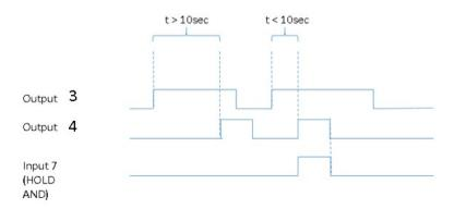
In our example, if output 3 is turned on, and then output 4 is turned on inside 10 seconds, the input 7 will become active.
