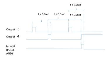
Input 8 remains on until the specified time has elapsed from the oldest activating output (unless pulse mode is selected, see below for details). In our example, when 10 seconds has elapsed from output 3 activation, the input 8 will be turned off.
