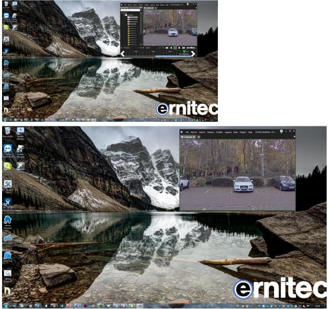
This is especially useful if the window auto-hide feature is used. The camera window can now be arranged to appear full-screen when in a small individual window. Such individual windows can also be tiled on the screen, giving 4 different EasyView windows appearing as a camera grid. This makes it possible to have multiple playback times on the same monitor.
