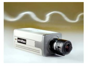
The EIP120 cameras can be used with standard lenses with either manual, video or DC iris. The cameras also have DIP-switch controlled functions including backlight compensation, auto white balance, auto gain control and flickerless for different application conditions.
