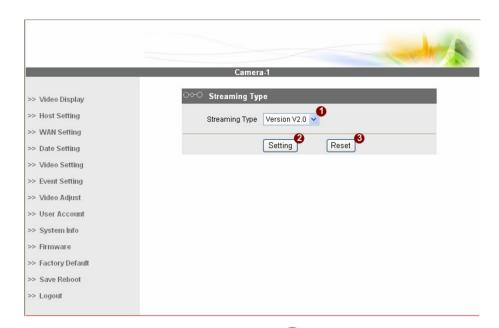
• STEP2: Select streaming protocol 1 [Version V1.0] (without audio function) or [Version V2.0] (with audio function), and click 2 [Setting] button to config settings, or 3 [Reset] button to re-enter the parameters. Configure these settings with reference to the table below. If you are still unsure what to set, contact your system administrator.
