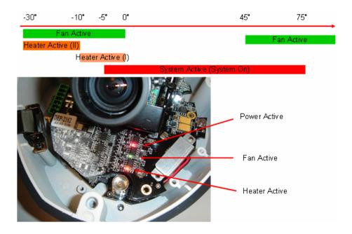
**NOTE:** Temperatures indicate here is spec for internal IC temperature, not for operating temperature.
