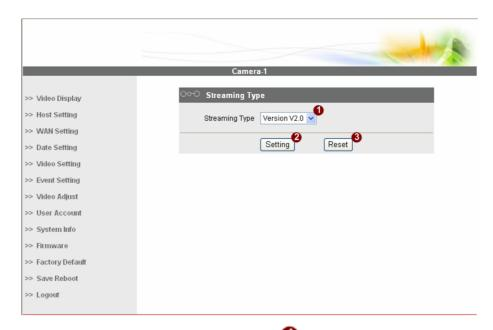
• STEP2: Select streaming protocol • [Version V1.0] (without audio function) or [Version V2.0] (with audio function), and click • [Setting] button to config settings, or • [Reset] button to re-enter the parameters. Configure these settings with reference to the table below. If you are still unsure what to set, contact your system administrator.
