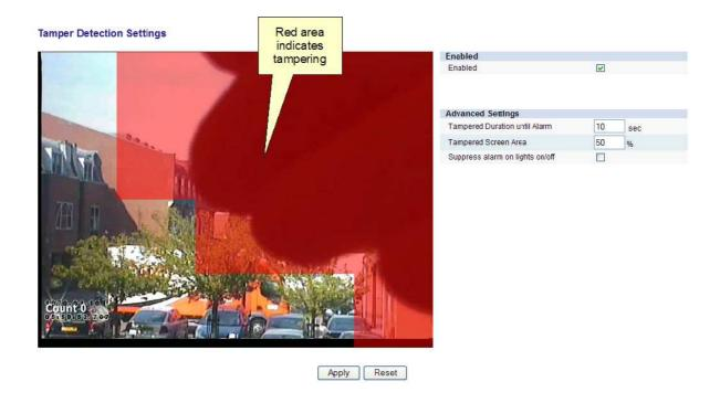
On the image display one can see the output of the tamper detection algorithm as red blocks on the image. The red area is where the algorithm has detected that the image has changed from its reference image. Once enough of the image has changed and remained so for a certain length of time, a tamper alarm is triggered.
