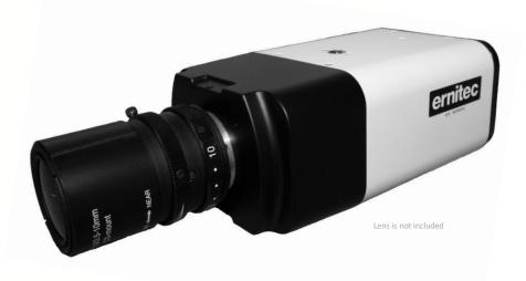
The Ernitec SX 602 cameras simultaneously offer High Definition megapixel resolution in 1080p format along with H.264 and MJPEG compression streams in real time .
