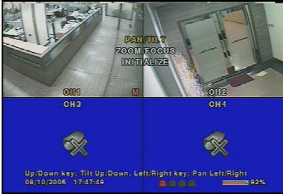
Figure 4.3.1. PTZF control screen
