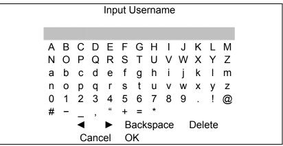
The next step is to enter a corresponding password. The preset password for "admin" is "1234", and the password "4321" is for "user".
