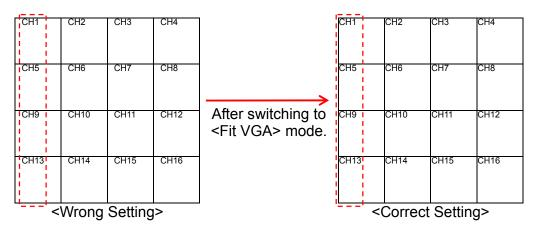
PC Monitor is used in the example above. In the <Wrong Setting>, the Title Position is set to <Fit BNC> instead of <Fit VGA>. Since it is not the right setting, the titles of CH1, CH5, CH9, and CH13 are slightly shifted toward the center screen of each channel. After switching to <Fit VGA>, the titles have been shifted back to the proper position as shown in the <Correct Setting>.
