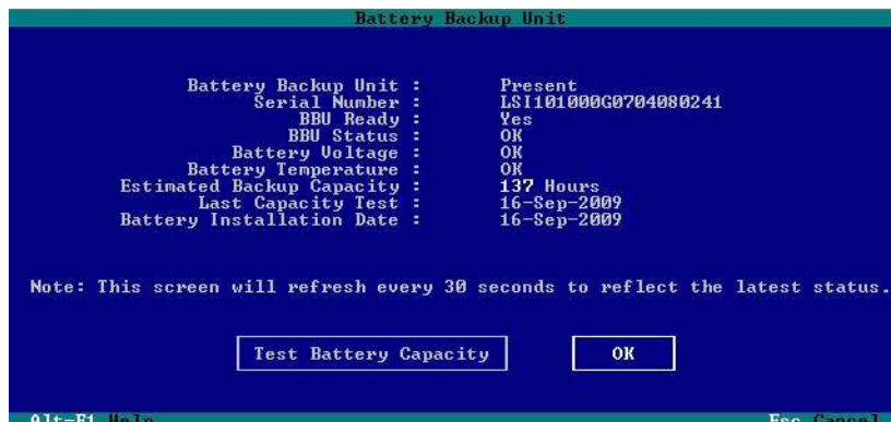
Figure 86. Battery Backup Information Screen in 3BM
