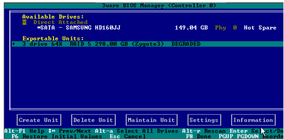
Figure 75. Degraded RAID 5 Array to be Rebuilt
