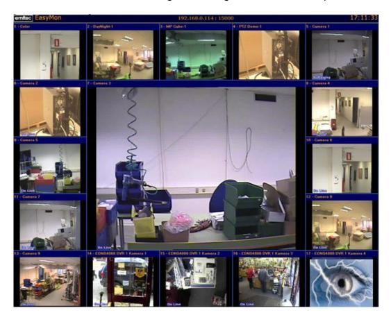
EasyMon combined with EasyView makes a virtual matrix. EasyMon has multiple split formats of 1, 4, 6, 8, 9, 10, 13, 16, 17, 21, 28, 25, 33 & 36 way split options. It supports live view and playback from multiple EasyView™ control stations all on the same network. The maximum live view screen split at D1 25fps is 36 way.
