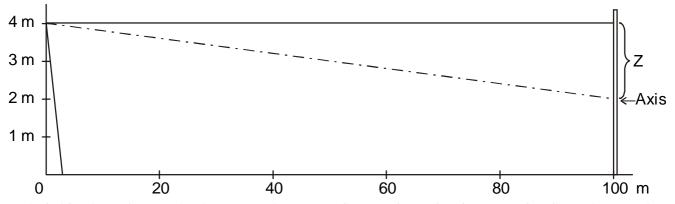
Typical side view of a terminating screen in 100 m distance from the detector. The dimension  $_{\pi}Z^{\pi}$  is app. 2.0 m corresponding to the value of the table in section 5.
