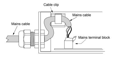
**Warning:** Before connecting the unit to the mains outlet make sure that the mains voltage change-over switch is set for correct mains voltage in order to avoid damage on the equipment. **Warning:** Make sure the equipment is earthed; otherwise the over voltage protection will not work! Although both the transmitter and the receiver are earthed no ground loop problems will occur due to the galvanic separation of the video signal introduced in the transmitter.
