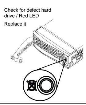
The machine is running but can hear a failure
